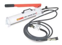
release operation to avoid damage to the pipe, and one pump can be used for two tools. All hoses supplied are 2-ply, 1/4" I.D. reinforced with two braids of high tensile steel wire and have a 20,000 PSI burst rating with an oil and weather resistant rubber coating.
