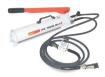
release operation to avoid damage to the pipe, and one pump can be used for two tools. All hoses supplied are 2-ply, 1/4" I.D. reinforced with two braids of high tensile steel wire and have a 20,000 PSI burst rating with an oil and weather resistant rubber coating.
