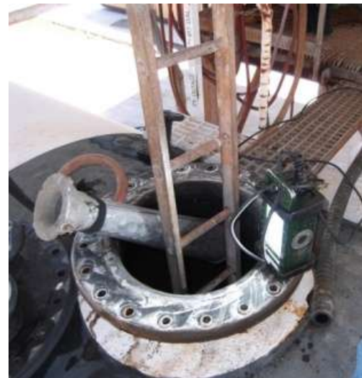
The BRICK™ Hung by Rope into Tank Car
