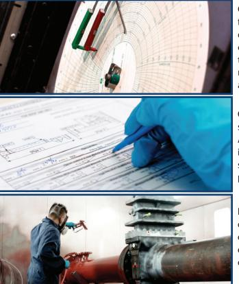
Our comprehensive **Quality Management System** includes full function, hydrostatic and pneumatic pressure testing to prevent defective orifice fittings from reaching service. Standard testing comes at no extra charge and includes verifiable pressurization to 150% of working pressure. Additional inspections, such as radiography, ultra sonic and liquid dye penetration - are also available.
