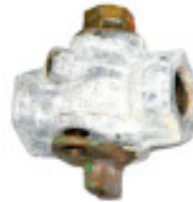
Galvanized plug after 30 hours
