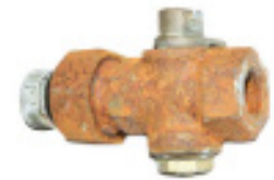
Cast iron plug after 12 hours
