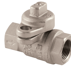
Tea treated valve after 250 hours
