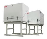
This enclosure allows the mounting of an NGC directly on the pipe in colder climates (ambient temperatures 0°F to -40°F). This weatherproof, insulated enclosure has brackets for the GC and the small start up/calibration bottle. It also has a removable plug that allows installing the enclosure over the probe so that the entire sampling system is heated to prevent liquid condensation of the sample prior to analysis.
